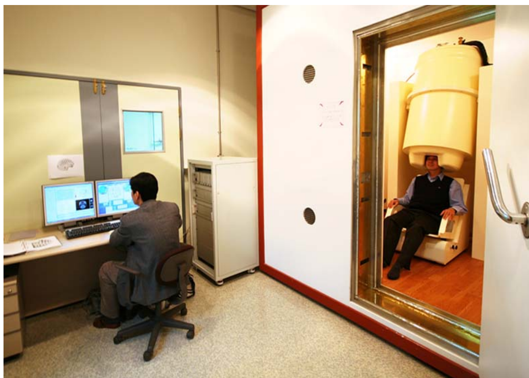
Figure 1. Magnetoencephalograph (MEG) system. A helmet-shape SQUID sensor array is located in a magnetically shielded room.
