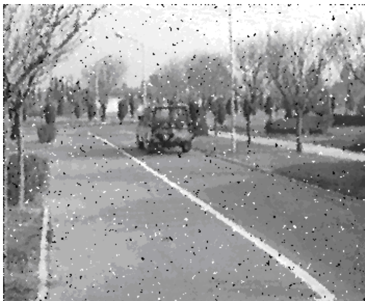
Figure 5(d). Filtered frame 335 of moving Patrol after applying CWM filter using N=3 frames under 50% noise density
