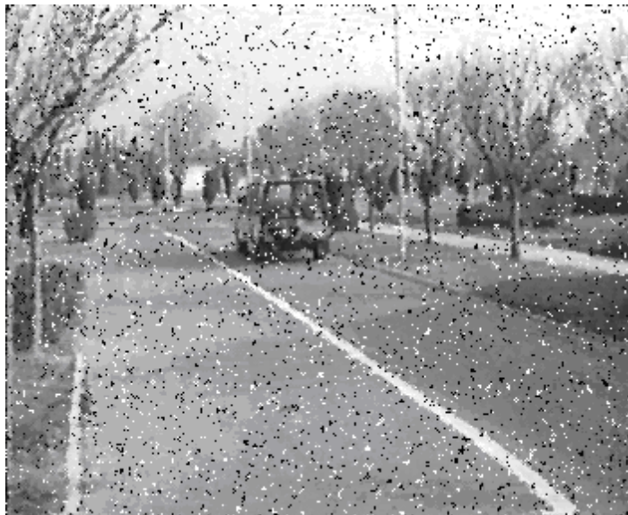
Figure 5(c). Filtered frame 335 of moving Patrol after applying CM filter using N=3 frames under 50% noise density
