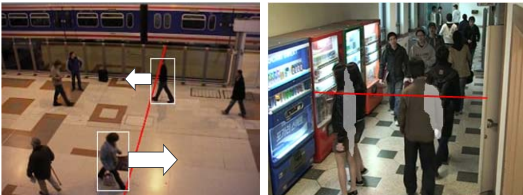
(a) (b) Figure 7. Difficulties in estimating object size: (a) size variation and different moving speed; , (b) occlusion between people
