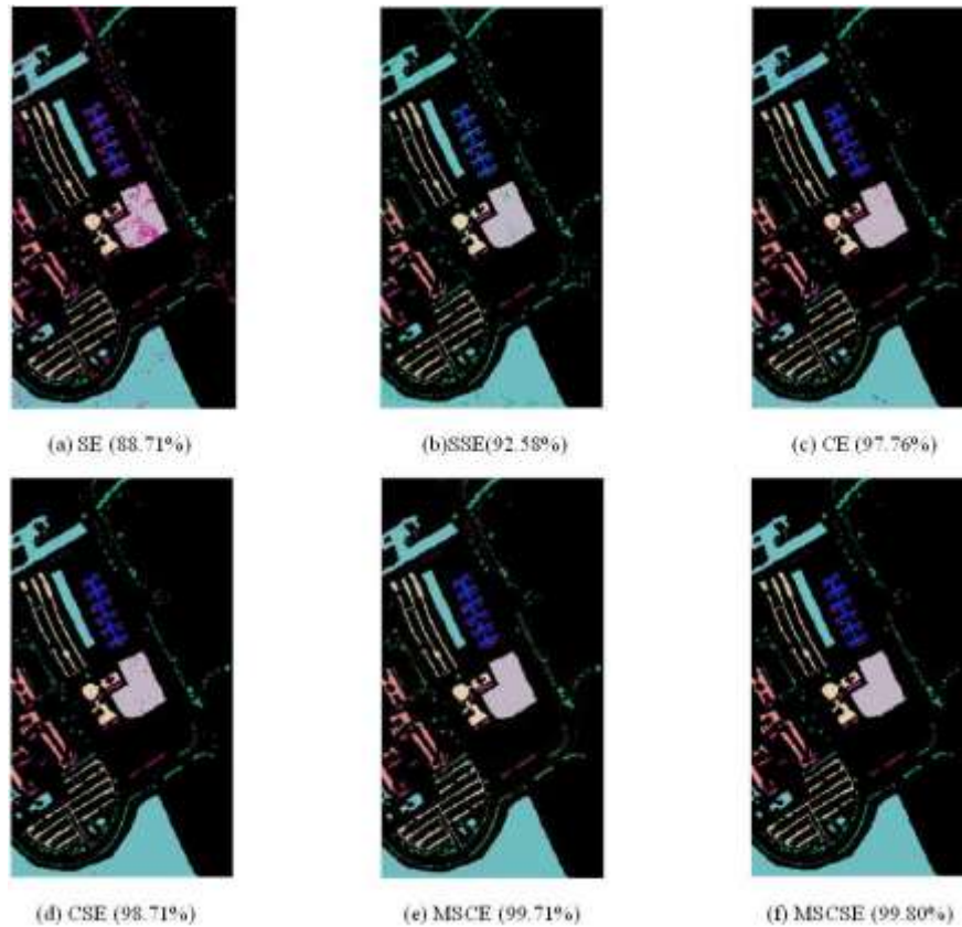
Figure 9. Classification Results of Different Classification Methods of ROSIS Data under the Condition of 10 Training Samples per Class
