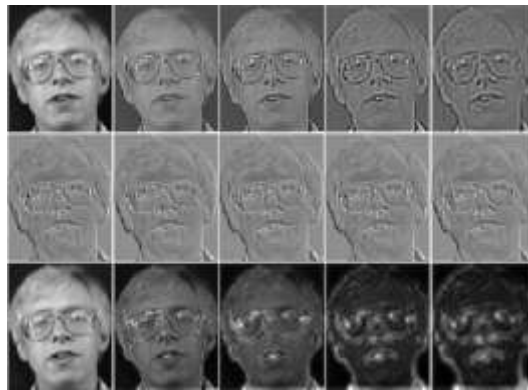
Figure 4. The Corresponding Mean Images to the Three Types of Gabor Kernel on One Face Image under Different Scales
