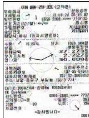
Figure 3. Key Points and Feature Vectors Extracted by SIFT
