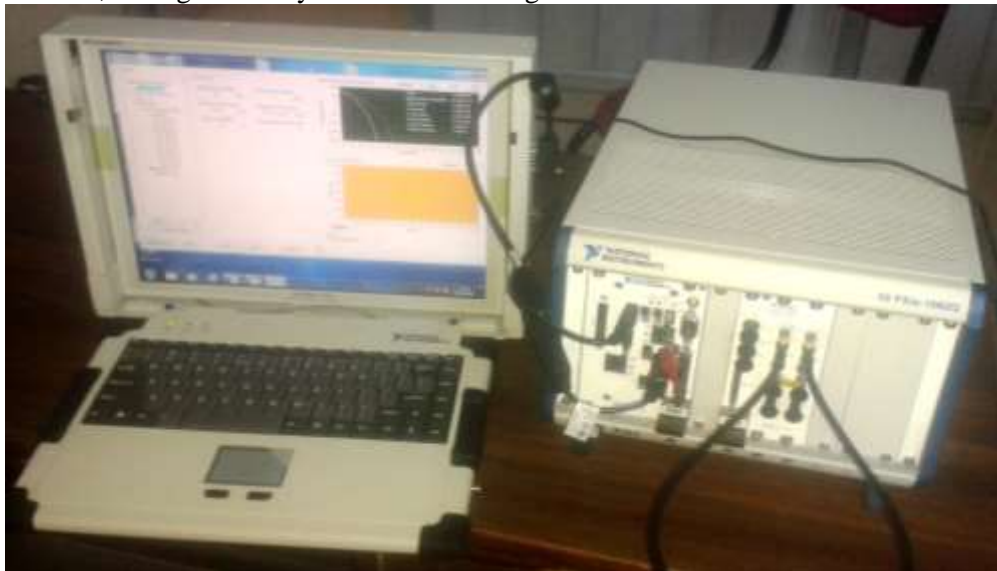
Figure 1. Experimental Set-up for WCDMA Link Based on NI Vector Signal Transceiver 5644R (Set-up & Experiment Conducted at Center of Excellence- R & D Wing, ACET, Amritsar)
