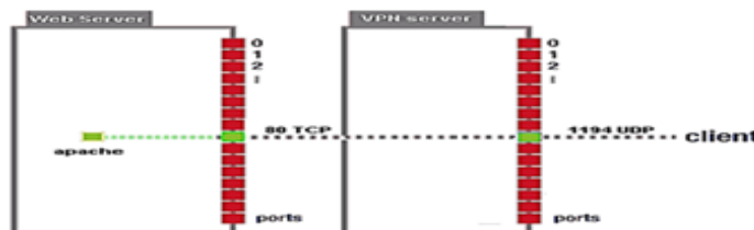
Figure 1. Typical VPN Mode - Client to Server Connection
