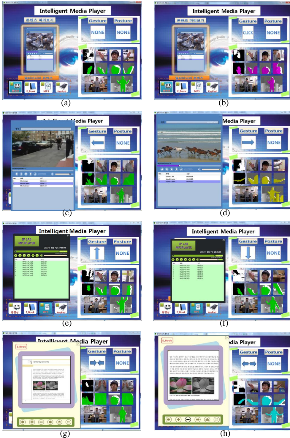
Figure 8. Gesture Recognition for Controlling System: (a) GUI, (b) “Click” Function, (c) Leftwards for “Previous”, (d) Rightwards for “Next”, (e) Upwards for “Volume on”, (f) Downwards for “Volume down”, (g) Zoom out, (h) Zoom in
