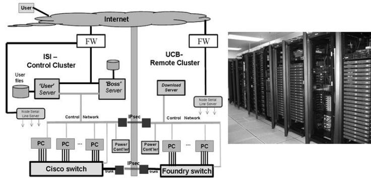
**Figure 1. DETERlab Test Bed**
