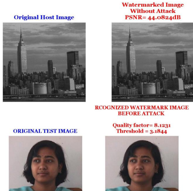
Figure 2. Original Host and watermarked host without attack with PSNR = 44.08 dB and face image whose features are embedded and recognized face image
