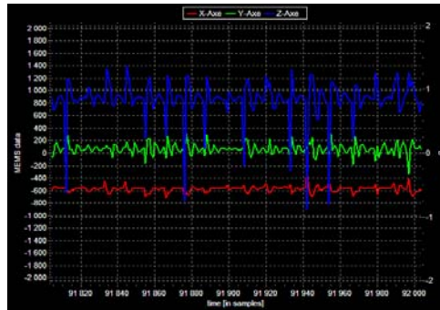
Figure 4. Experiments with accelerometer (acquired during fine shaking of camera)
