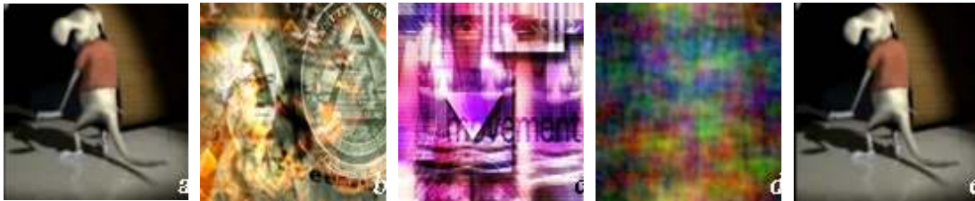
Figure 7. Encryption and decryption color image: (a) target image, (b) key image 1, (c) key image 2, (d) encrypted image, (e) decrypted image.
