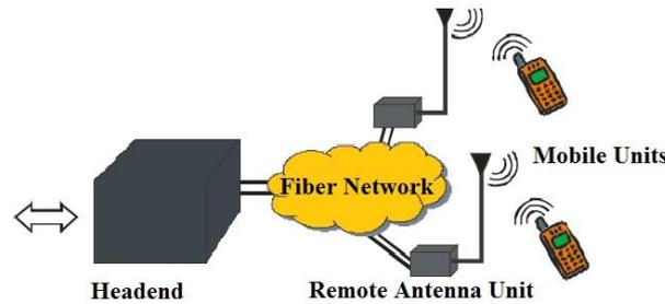
**Figure 1. Radio over Fiber System Concept**
