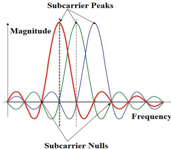
**Figure 3. OFDM Multicarrier System**
