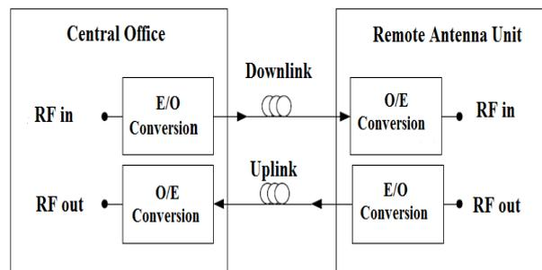
**Figure 2. Radio Over Fiber System Architecture**
