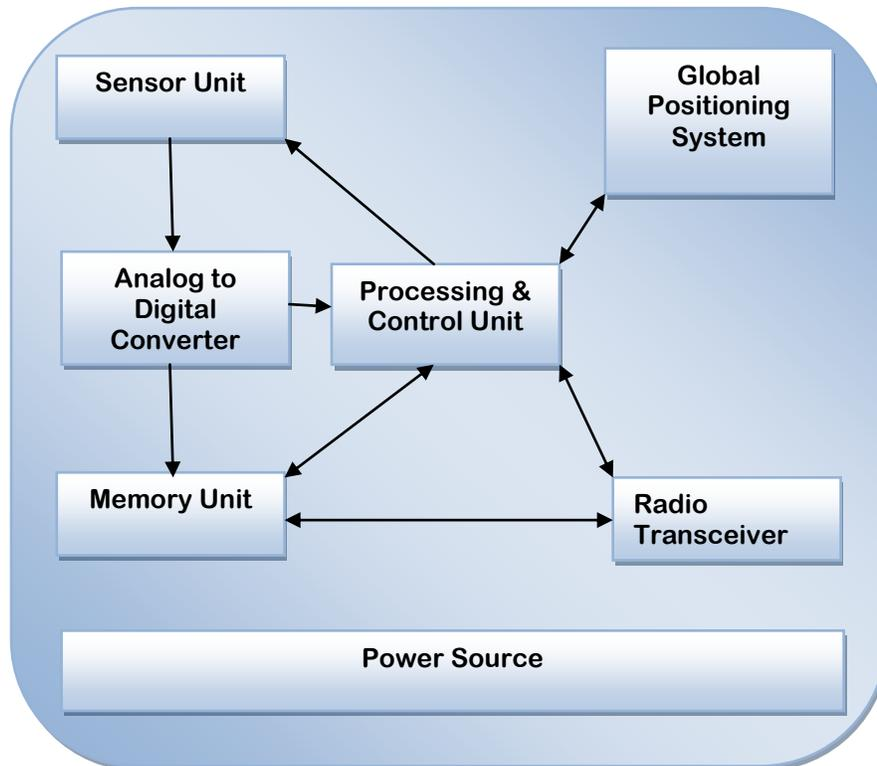
**Figure 1. The Block Diagram of a Sensor Node**
