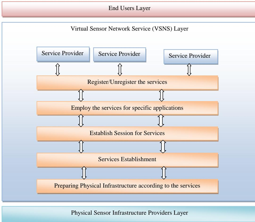
**Figure 5. Layered Architecture for Service Provisioning**
