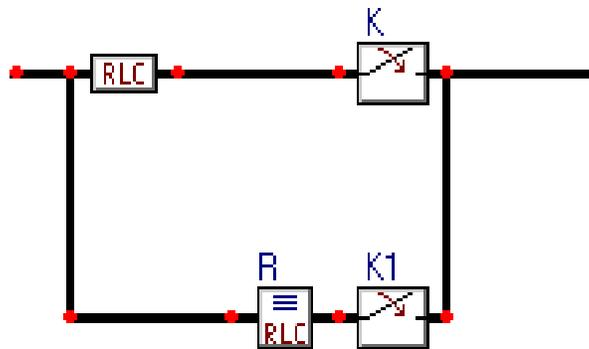
Figure 5. Circuit Breaker Attached Additional Single Stage Closing Resistors
