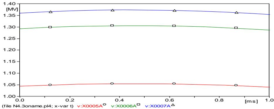
**Figure 12. The VFTO Waveform (Additional 400 Ω Multistage Closing Resistors)**
