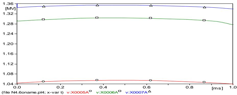
**Figure 15. The VFTO Waveform (Additional 400  $\Omega$  Multistage Closing Resistors and Lightning Arresters in Two Terminals and the Middle of Lines)**
