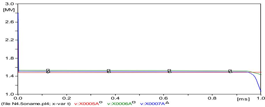
**Figure 14. The VFTO Waveform (Lightning Arresters in Two Terminals and the Middle of Lines)**
