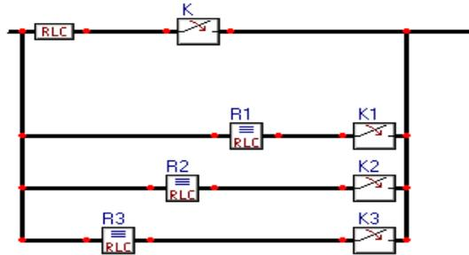
**Figure 6. Circuit Breaker Attached Additional Multi-Stage Closing Resistors**
