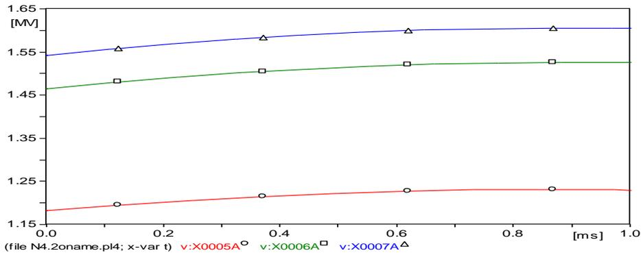
**Figure 11. The VFTO Waveform (Additional 100 Ω Single Stage Closing Resistors)**
