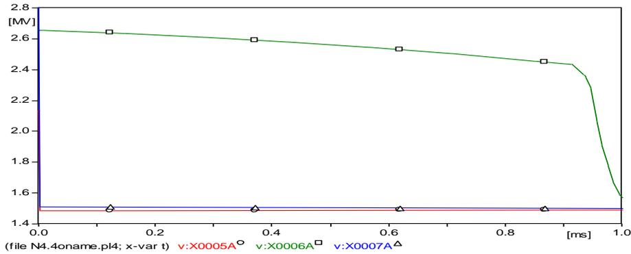
**Figure 13. The VFTO Waveform, (Lightning Arresters in Two Terminals of Lines)**
