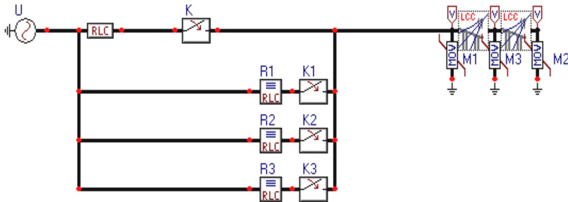
Figure 9. ATP-EMTP Simulation System Model
