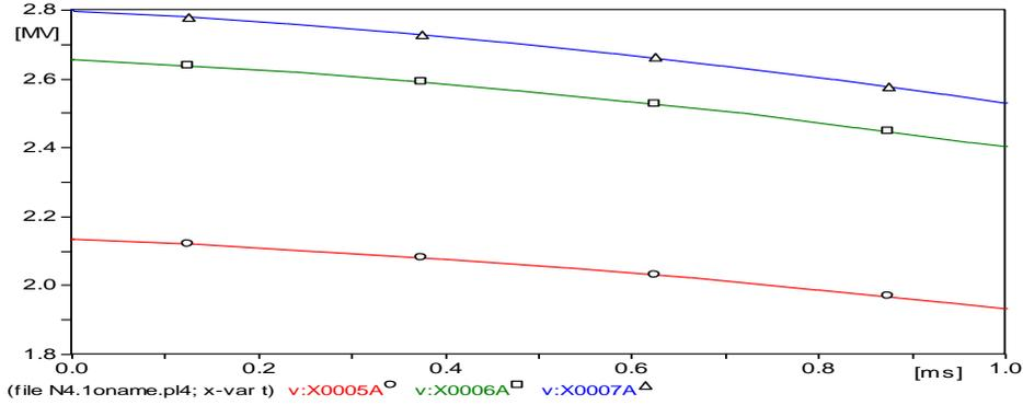
**Figure 10. The VFTO Waveform (No Additional Closing Resistors and Lighting Arresters)**
