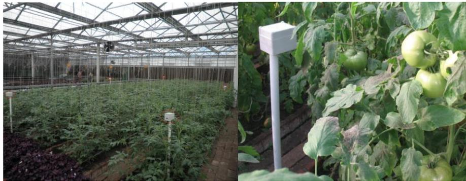
**Figure 2. The Sensor Nodes Deployed in the Greenhouse**
