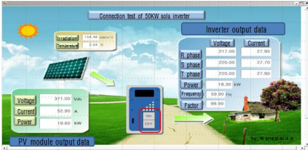
Figure 7. Monitoring Panel using HMI S/W
