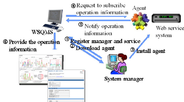
Figure 1. Web Service Monitoring Process
