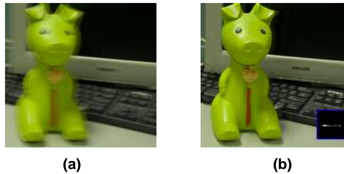
Figure 7. Image captured with hand held camera (a) Blurred image due to camera shake and (b) Blind deconvolution result [23]
