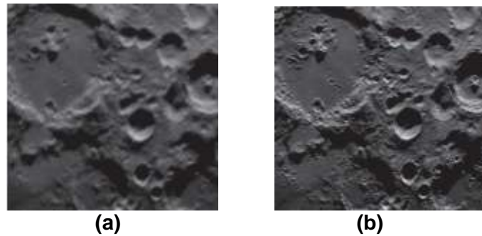
Figure 9. Moon Surface video distorted by atmospheric turbulence (a) One Observed Frame and (b) Blind Deconvolution result [3]
