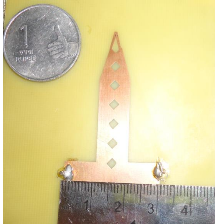
Figure 6. Fabricated Prototype of Grooved Microstrip Band Pass Resonator Filter on FR4 Substrate (Horizontal Measurement)
