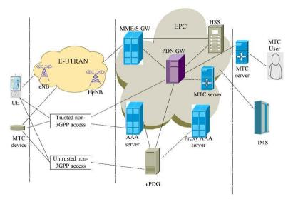
Figure 2. Network Architecture of LTE
