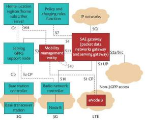
Figure 1. The Architecture of Evolved Packet System
