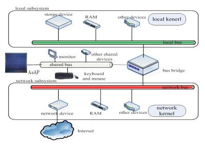
Figure 3. The New High Security Computer Architecture
