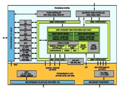
Figure 1. Zynq-7000 System Structure Block Diagram
