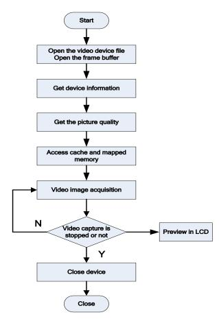
Figure 3. Flow Chart of Image Acquisition via V4L2
