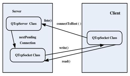
Figure 4. QT Network Programming Block Diagram
