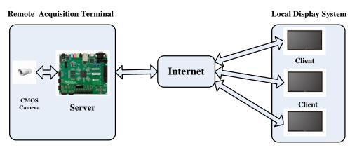
Figure 2. Embedded Network Video Monitoring System Block Diagram
