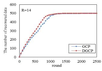
Figure 5. Data Collection Process using GCP and DGCP in Dense Networks (Centralized Disaster Networks)
