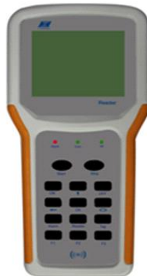
Figure 6. JRFR-2-21 (900M) Wireless Receiving End Humiture Recorder
