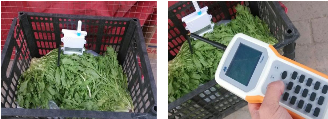
Figure 8. The Individual RFID and Receiving Recorder Put in the Holding Room
