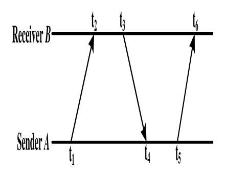
Figure 3. A Sender A-receiver B Two-way Timing Exchange Model
