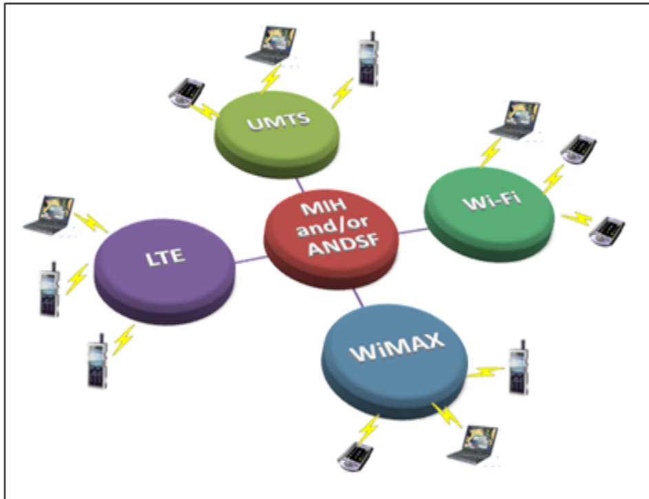
Figure 1. Various Radio Access Technologies (RATs) Integration Supported by MIH/ANDSF
