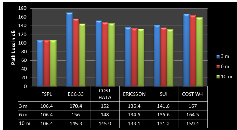
Figure 4. Analysis of Simulation Results in Urban Environment at a Reference Distance of 2 km for Different Receiver Antenna Heights
