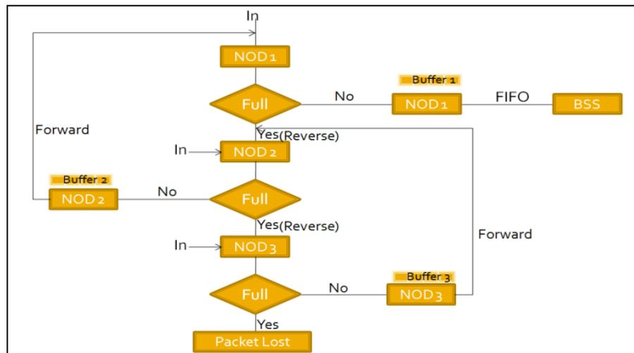
**Figure 1. Flowchart of Buffer Management Process. Consider the case where the first wireless node to receive packets. If buffer in node 1 is empty, the packet is forwarded into the queue**
