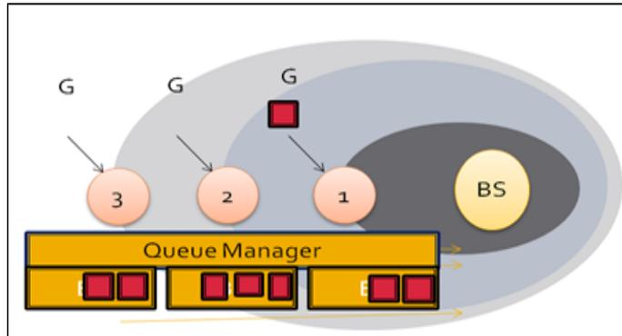
**Figure 2. Node Chain Topology; Topology being used is formed of 3 nodes and 1 base station**
