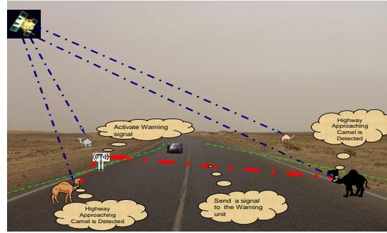
Figure 2. The Warning System being Activated as Camels approach the Highway.
