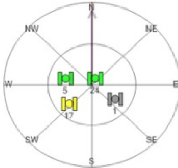
Figure 4: Graphical Representation of a $GPGSV Sentence, Where the Center of the Circle Marks the Current Position and the Edge of the Circle Marks the Horizon.
