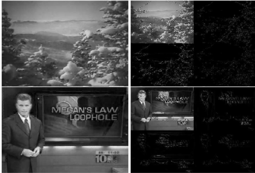
Figure 3. Wavelet Decomposed Images: Image on the right is decomposed version of the image on the left.
