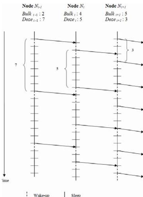
Figure 1. Sleep and wake-up states of sensor nodes in LMAC protocol
