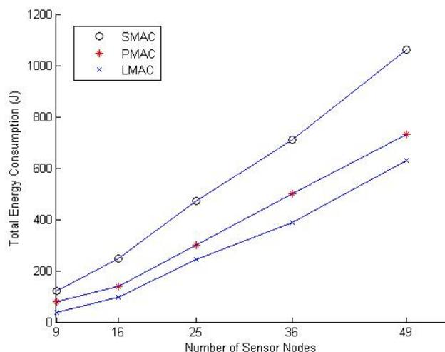
Figure 4. Total energy consumption under different numbers of sensor nodes
