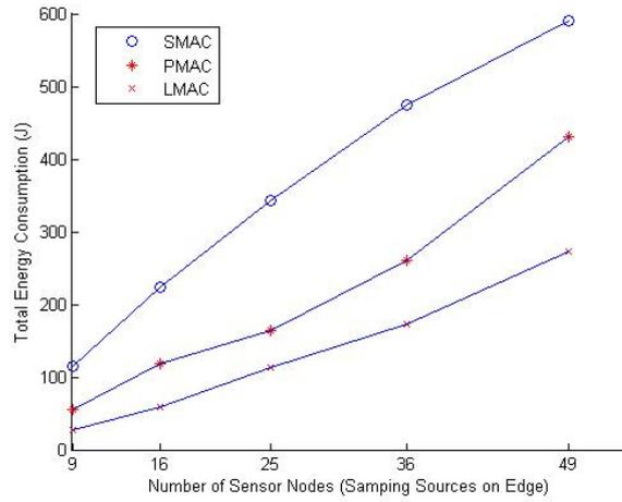
Figure 5. Total energy consumption under different numbers of sensor nodes & Source Nodes on Edge
