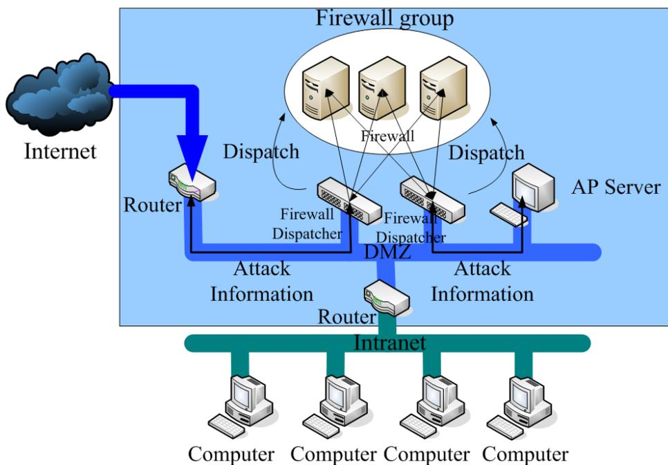
Figure 1. Structure of conventional Firewall scheme
