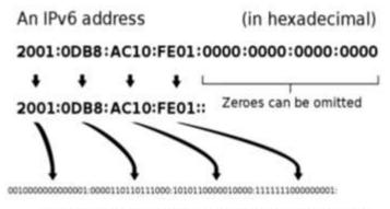
Figure 1. An IPv6 Address Representation
