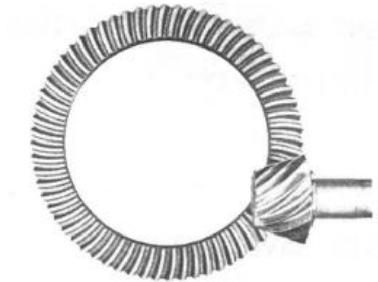
Figure 5. Hypoid Gear Machining Simulation
