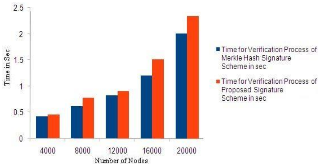
Figure 4. Graphical Representation of Performance Analysis of Time Required for Verification Process for Merkle Hash Signature Scheme & Proposed Signature Scheme in Sec. for different of Nodes
