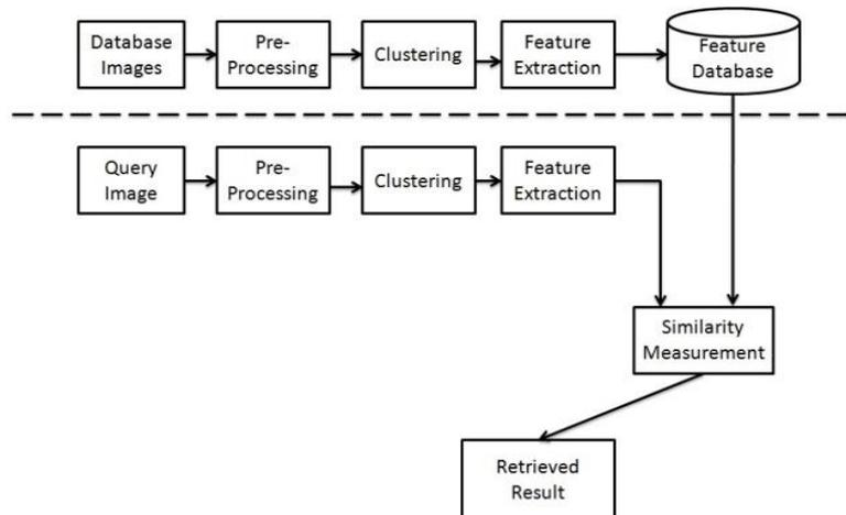
**Figure 1. Content Based Image Retrieval Model**
