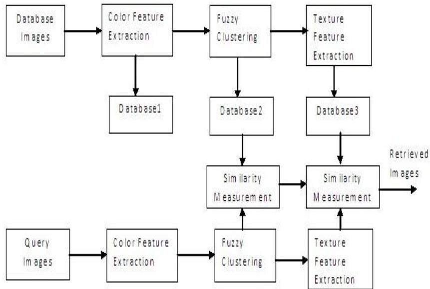
**Figure 4. Architecture of Proposed CBIR System**
