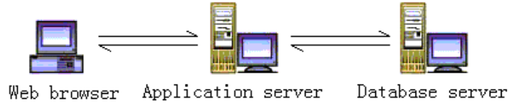
Figure 2. ADO Three Layer Structure
