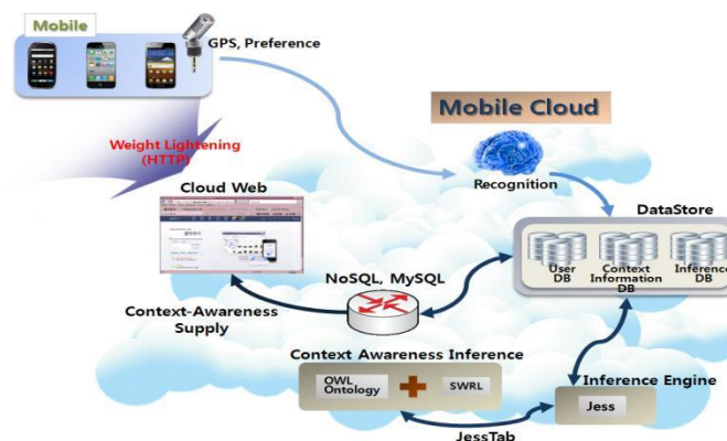
Figure 1. It is the System Overflow Chart. It Provides Situation Awareness Service through Jess Inference Engine and NoSQL by Receiving Situation Inference Data from Mobile Devices
