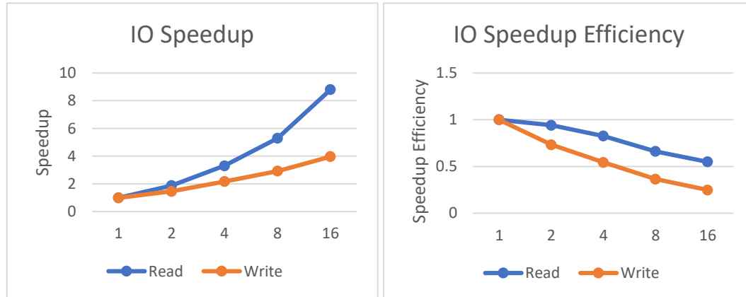
Figure 7. The Speedup and Speedup Efficiency of Reading and Writing Performance of the Cloud Storage for Seismic Big Data
