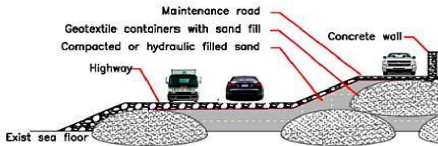
Figure 4. Construction of Dike
