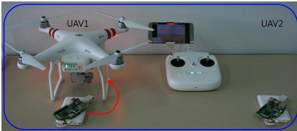
Figure 5. The Transmission Module that will be attached to the UAV
