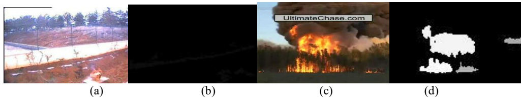
(a) the key frame of flame video; (b) the corresponding flame texture feature map; (c) the key frame of flame video; (d) the corresponding flame texture feature map.
