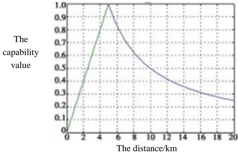
**Figure 1. The curve of the Capability Function of UAV**
