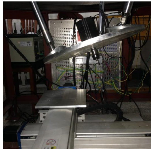
Figure 14 The Cutter, the X-Y Table and the Synthetic Trajectories
