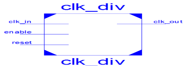
Figure 10. Divide By 2 Counter
