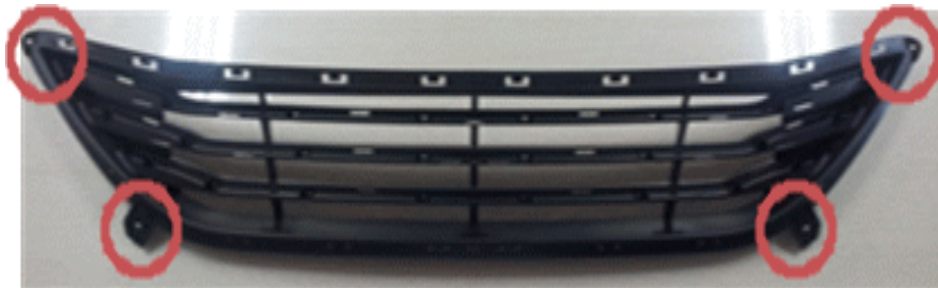
Figure 1. The Four Areas of High Failure
