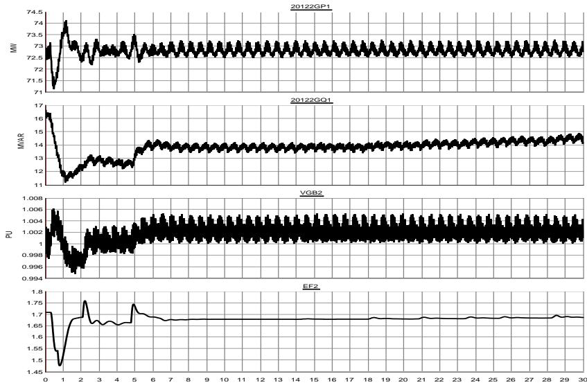
Figure 6. Variations of Real Power, Reactive Power, Terminal Voltage and Excitation Voltage of Northern Generator.
