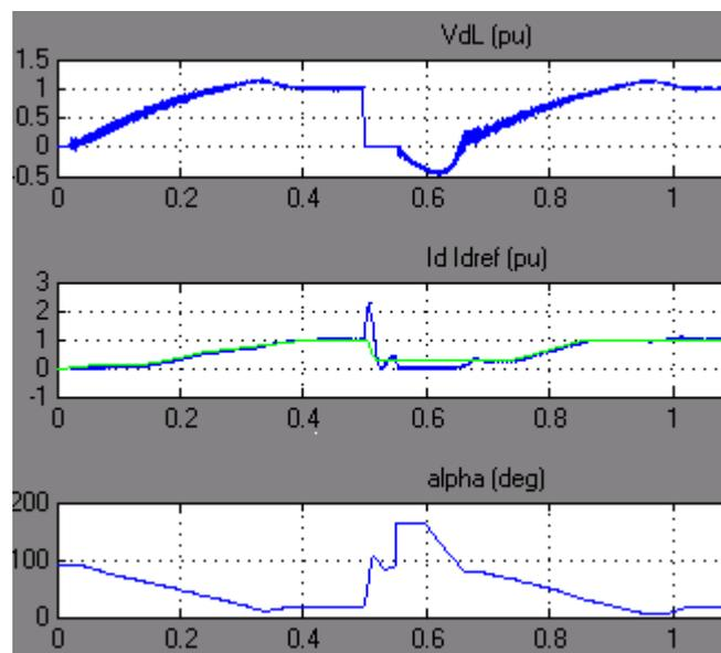
**Figure 3. Side of Rectifier Dc Line to Ground Fault Simulation Results**
