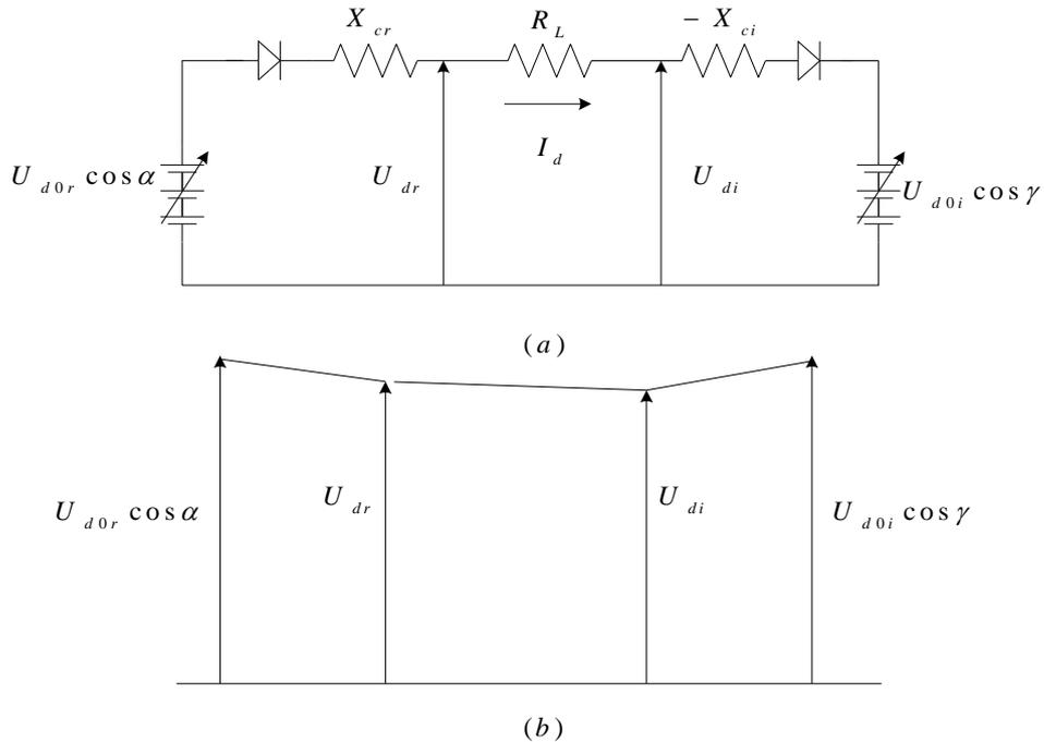
**Figure 1. High Voltage Dc System Transmission Link (A) the Equivalent Circuit; (B) the Voltage Distribution**
