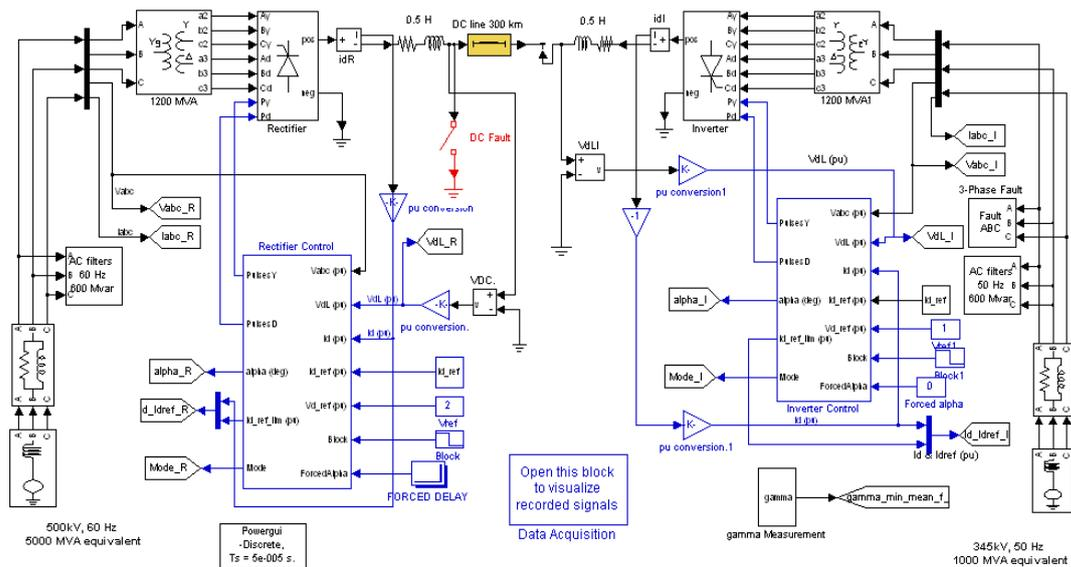
**Figure 2. Twelve Pulse HVDC Power Transmission System**
